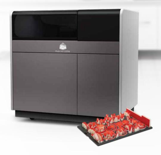
3D Systems' comprehensive MultiJet Printing solution for jewelry casting includes the ProJet MJP 2500W 3D Printer, software, and materials to quickly and consistently generate micro-detail, precision, 100% wax sacrificial casting patterns for high capacity jewelry production. Eliminate tooling time, cost or geometric limitations, and deliver reliable and repeatable direct casting efficiency.
